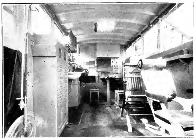
INTERIOR OF A FRENCH DENTAL AMBULANCE. THIS IS A ROLLING DENTAL OFFICE, COMPLETELY FITTED AND MOUNTED ON AN AUTOMOBILE TRUCK.
